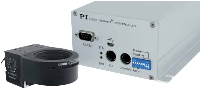
The microscopy package: Objective nanofocusing system with 1 mm travel range and adapters for M25 threads. The controller comes with an extensive software package e. g. for automation and also supports manual control via joystick
