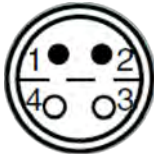
Figure 19: Sensor connection: LEMO connector FFA.0S.304.CLAC32Y, contact side
