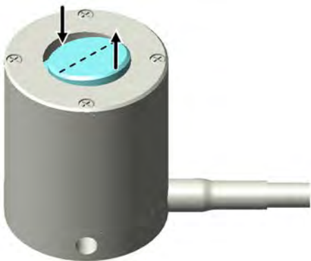
Figure 5: Maximum displacement in the positive direction of motion around axis 2. At the connected channel 2 of the amplifier, the output voltage U_{Piezo} is 100 V. The displacement shown is strongly exaggerated for better understanding.
