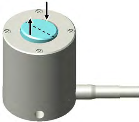
Figure 4: Maximum displacement in the positive direction of motion around axis 1. At the connected channel 1 of the amplifier, the output voltage U_{Piezo} is 100 V. The displacement shown is strongly exaggerated for better understanding.
