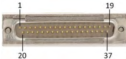
Figure 18: Sub-D 37 (m) piezo and sensor connection
